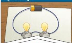
**Electricity can** only flow around a complete **circuit** that has no gaps. There must be wires connected to both the positive and negative end of the power supply/**battery**.
